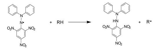
0.000625g of DPPH was dissolved in 25 ml of absolute methanol. 1990 µl of this solution was added to the 10 µl of plant extract. Before starting the readings, the UV spectrophotometer was set reading a blank with methanol solution only. The changes in the colour from deep-violet to light yellow were measured at 515nm for 20 minutes and the antioxidant activity percentages were calculated according to the equation
